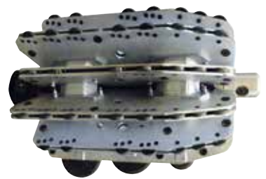
Roller cutter body with cutter strip Ø 1000 mm
